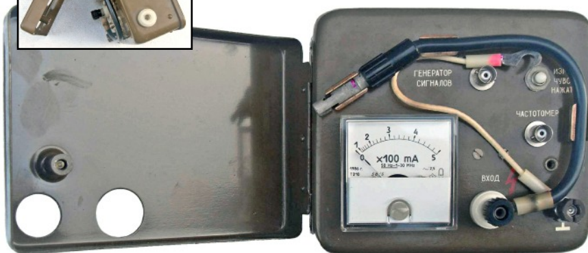
Dummy load with sockets for connecting a signal generator and frequency counter.
