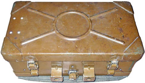
Powering the R-143 during longer and/or static operations a separate metal box with rechargeable batteries was used.
