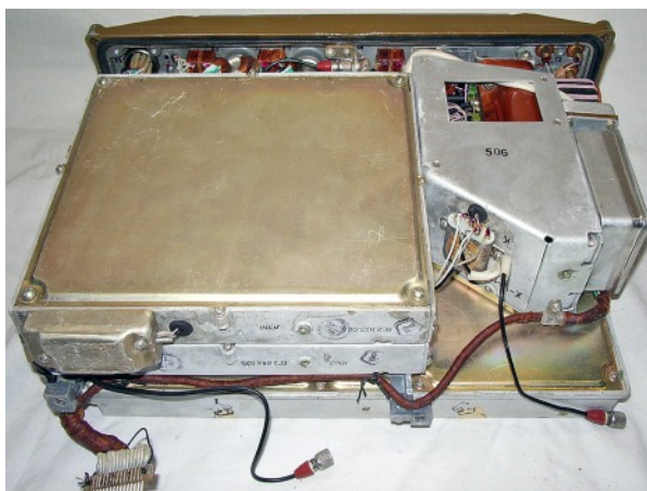
Internal view of the R-143 showing its modular construction.
