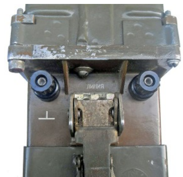
Right hand (part) side view showing sockets for connecting a field telephone.
